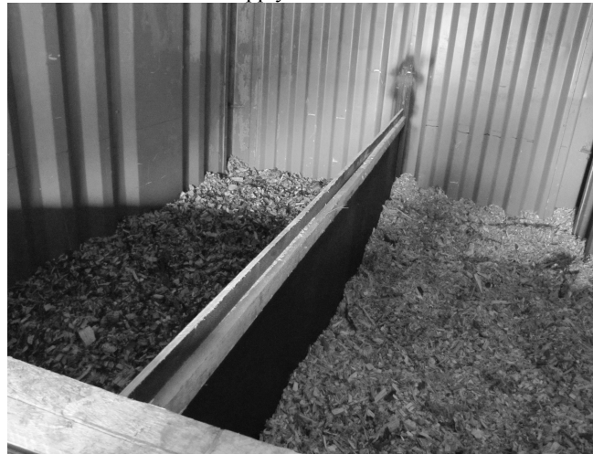
Figure 1. The drying chamber was divided in two to enable the simultaneous drying of two different wood chip types. (Photo: Jyrki Raitila)
