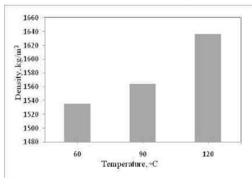
Fig 7: Density of geopolymer bricks at elevated temperature
