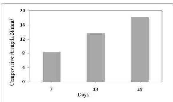
Fig 6 compressive strength of geopolymer bricks at water curing
