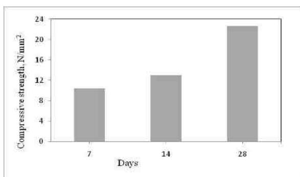
Fig 5: compressive strength of geopolymer bricks at room temperature
