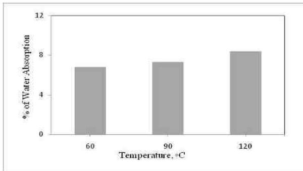
Fig 10: Water absorption of geopolymer bricks at elevated temperature
