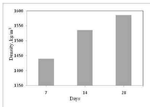
Fig 8: Density of geopolymer bricks at room temperature
