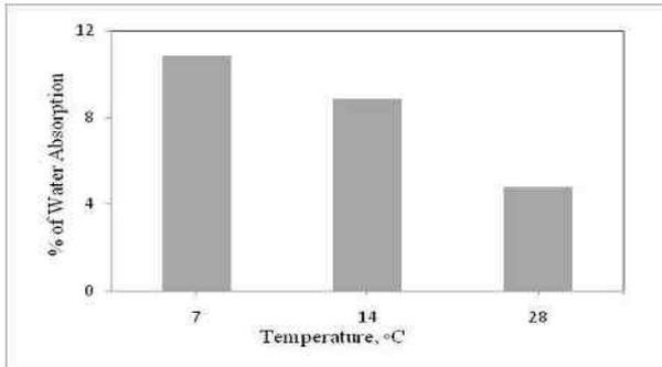
Fig 11: Water absorption of geopolymer Bricks at room temperature
