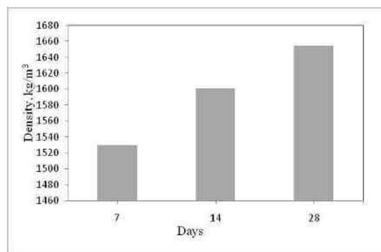
Fig 9: Density of geopolymer bricks at water curing
