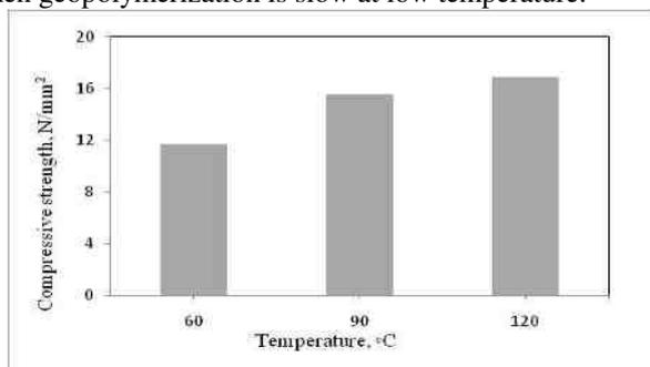
Fig 4: Compressive strength of geopolymer bricks at elevated temperature
