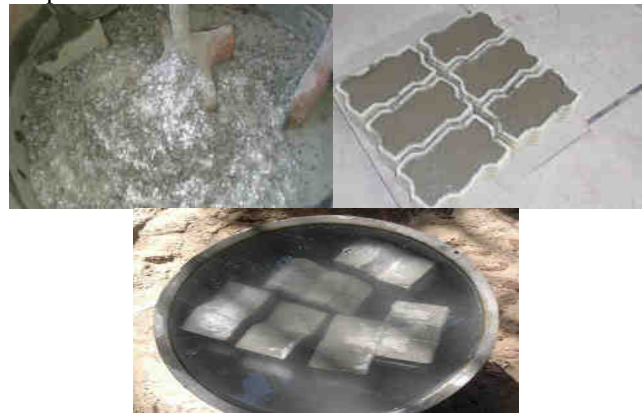
Fig 3: Mixing, Casting and Curing of Paver Block
