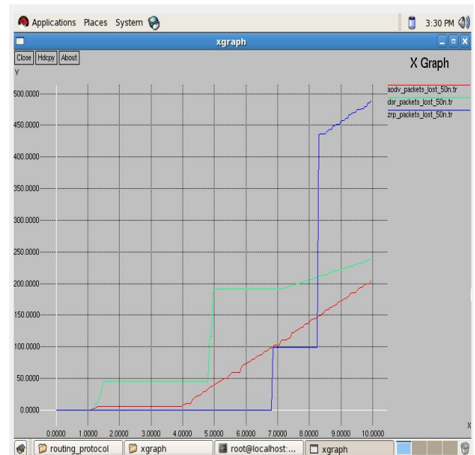
Fig 5.11: X-graph representing comparison of packet lost in simulation for AODV, DSR and ZRP.
