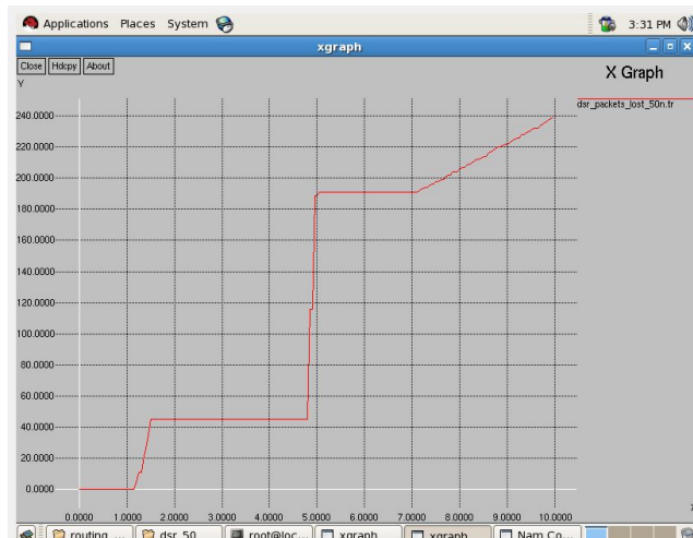
Fig 5.6: X-graph representing packet lost in simulation for DSR.
