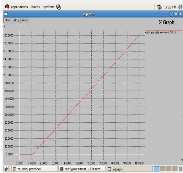
Fig 5.2: X-graph representing packet received in simulation for AODV.
