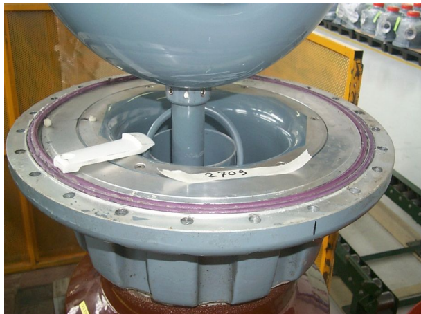
Fig. 5 Damage of SF6 insulation current transformer with the transport.
