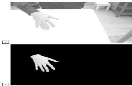
Figure 2: Figure (a) shows the human hand in a typical calibration phase. In figure (b) only that region got left, which represents the human skin color. These color samples are used for further operations, the calibration is complete.
