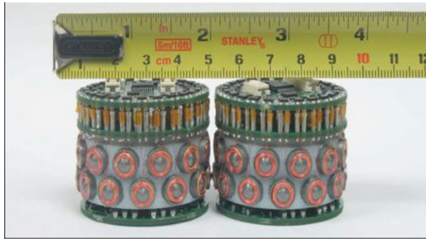
Fig1 Claytronics atom prototypes. Each 44-mm-diameter catom is equipped with 24 electromagnets arranged in a pair of stacked rings.
