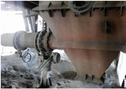
Photo2 – Motorized & Manual valves in cold air entry to ash cooler
