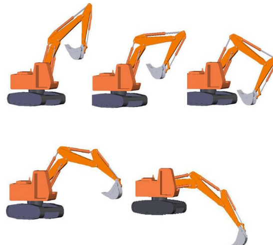
Fig.4 Second and third load conditions: lifting at the maxima and minima distance from axle of rotation.
