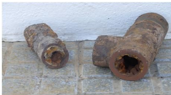
Figure 1: External and internal corrosion in iron pipelines (authors).
