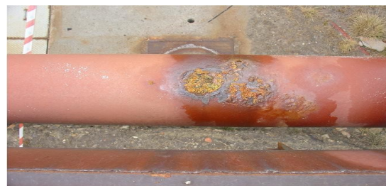
Figure 8: Pitting and metallic corrosion observed in pipeline to dose ferric chloride (authors).
