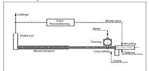
If production on the moulding line has to stop for a period of time, the critical stand-still time must be considered and the mould conveyor and synchronized belt conveyor should be emptied
