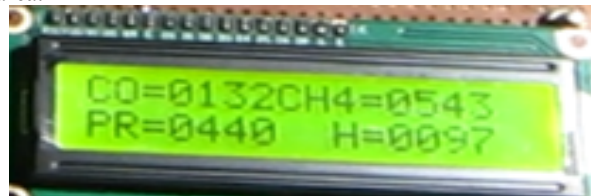
Figure 9: Displaying concentration of toxic and combustible gases
