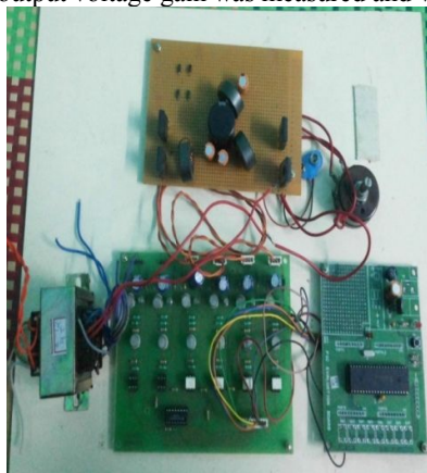
Figure 9 hardware circuit of ZVS half bridge DC-DC Converter
