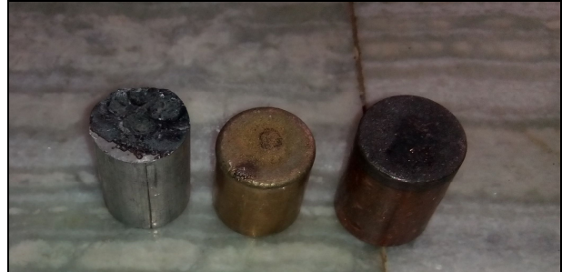
Fig.2:- Different Electrodes (copper, brass, aluminium)
