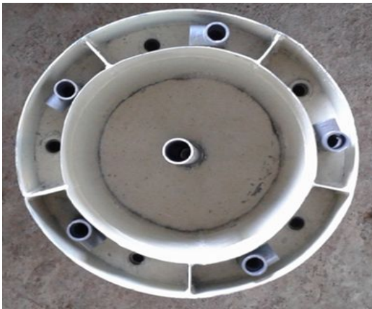
Fig: Inlet And Outlet Pipes
