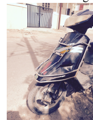
Fig. I: BLDC motor fitted in front wheel hub
