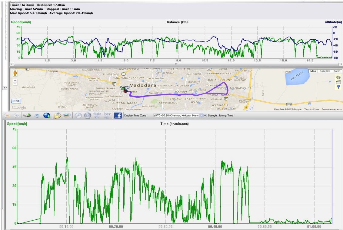
Fig VII: Data recorded by QStarz BT-Q1000eX GPS data logger in Gasoline Mode
