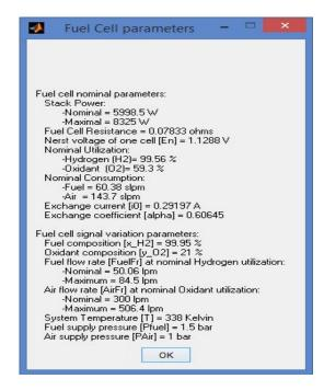
Here a 6 kW fuel cell stack is feeding a three phase load at 100 V. We used a 3 arm bridge MOSFET inverter to convert d.c. voltage into a.c. and a harmonic filter to reduce the harmonic content of the waveform. Then we used a three phase transformer to step up the voltage level to 100 V. Here we are using series R-L-C load.
