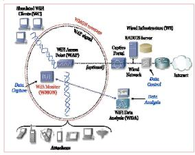
The above figure shows the architecture used in honeyspot.WAP which is in the middle is the wireless access point. It gives the wireless networks to the users for internet connection. Attacker can connect to it.
