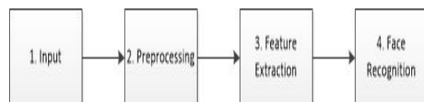
Figure 1 - Face Recognition Process
