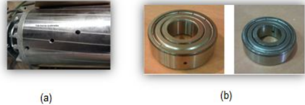
Fig. 6. Simulation of failures: broken bars (a); bearing inner and outer race (b).
