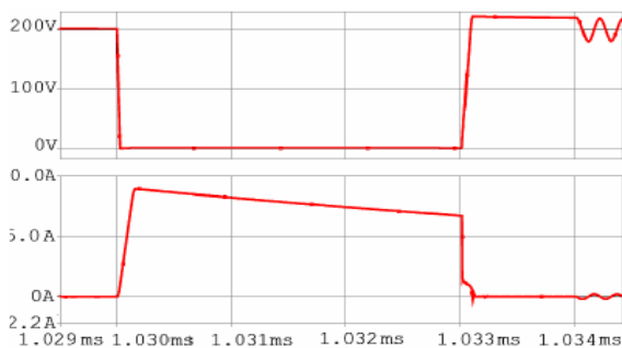
Figure 9. Top: switch S 3 voltage, bottom: switch S 3 current
