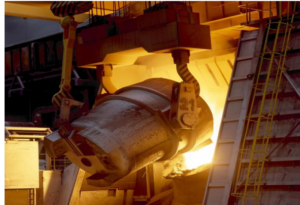
Fig 2 The process of pouring a hot metal by lifting it with the help of heavy cranes
