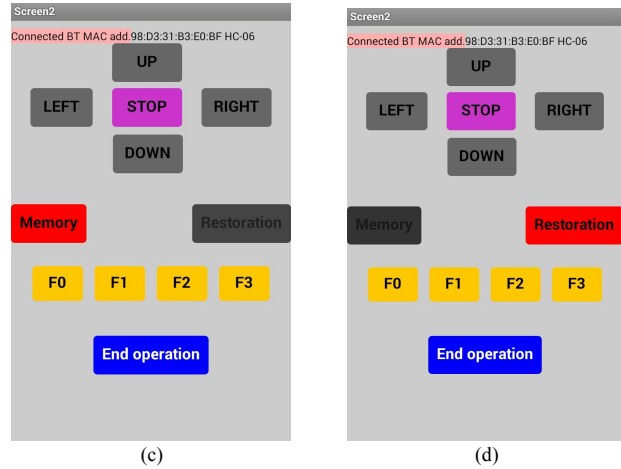
Figure 15. Different operating screens of the HMI (a) initial screen (b) three selection items (c) memory operation (d) restoration operation
