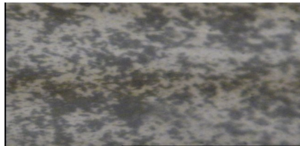
Fig 6: Optical Micro. [Al7075+1.5%SiC]
