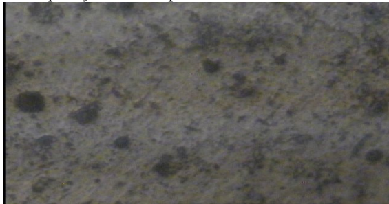
Fig 2: Optical Micro. [Al7075+0.5%SiC]
