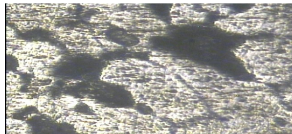
Fig 8: Optical Micro. [Al7075+2%SiC]
