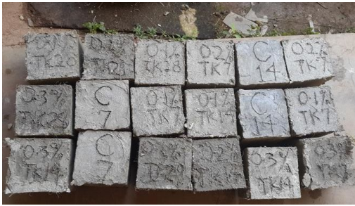
Figure 1: Concrete Cubes after Demoulding
