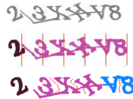
Fig.9: Successful segmentation produced by the proposed algorithm.
