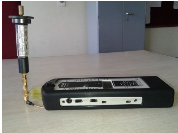
Fig. 3 Hf59b TM Device Used To Measure Radiation Levels
