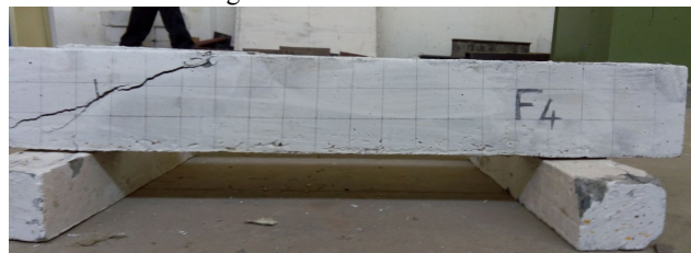
Fig 7 FRC at shear zone without web reinforcement.
