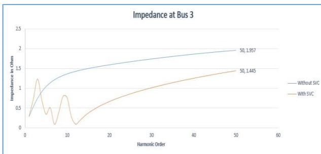
Figure 11: Impedance plot at bus-3 for with and without SVC.
