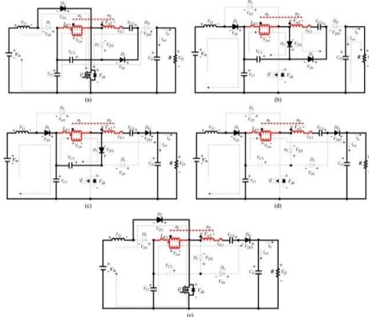
Fig.1.2. Equivalent circuits of five operating stages during one switching period at C-CCM operation
