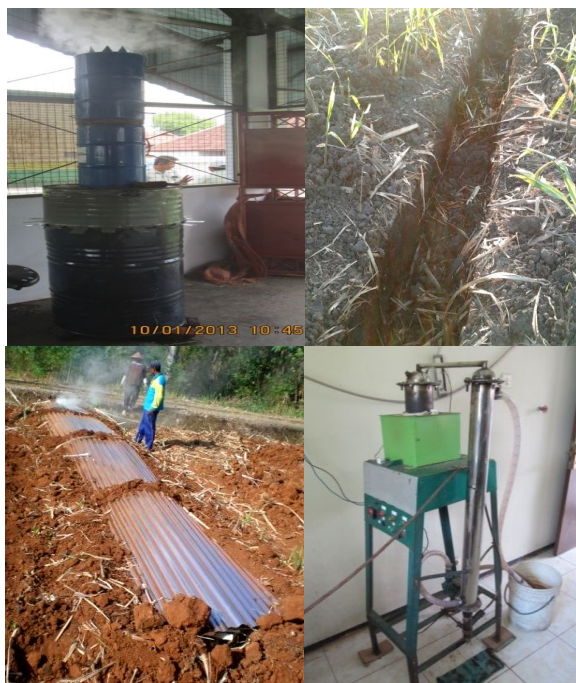
Figure 1. The techniques for making biochar: (a) drum kiln; (b) trench kiln; (c) mound kiln, (d) pyrolysis reactor
