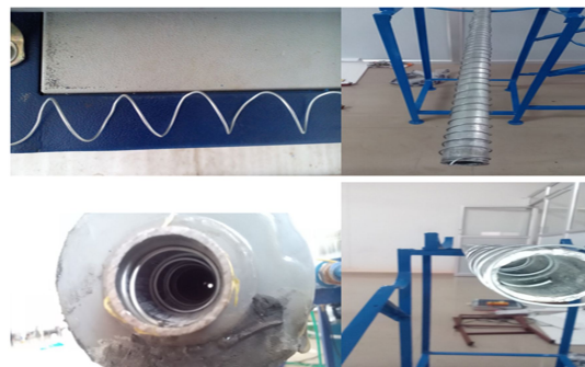
Fig 3 GI wire coil inserts used in the experiment, p = 30mm, l=1.4m
