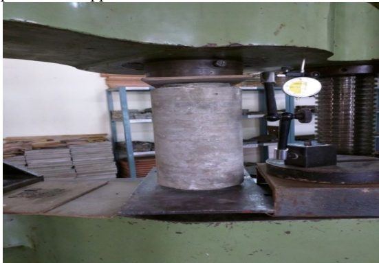
Figure 2 Experimental Setup of Column Specimens
