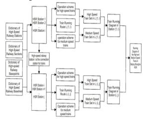
The structure of the running diagram of the high and medium speed trains in Beijing-Shanghai High-Speed Railway
