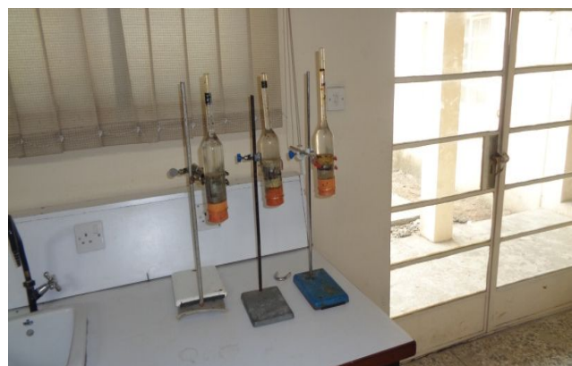
Figure 4: Experimental setup for imbibition occurring spontaneously in a system of oil/brine/reservoir rock
