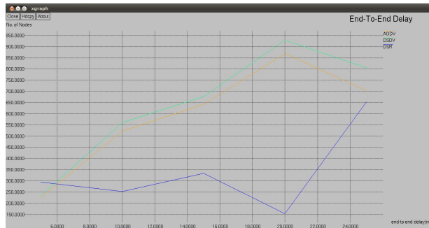
Fig. 15: End-to-End Delay for AODV, DSDV and DSR.
