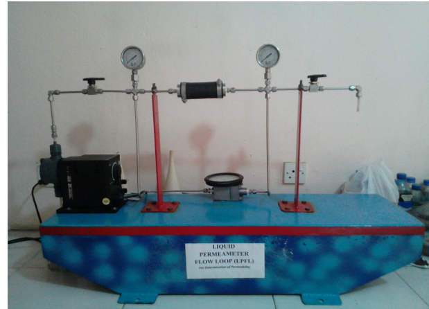
Fig. 2: Locally fabricated permeameter for shale permeability determination
