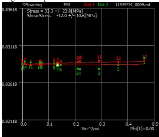
Graph. 4 d spacing versus \sin^2\psi values of annealed sample
