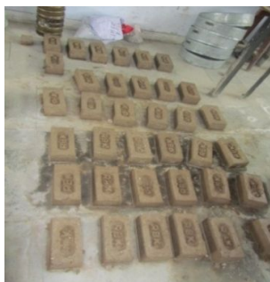
Figure2: Demoulding of bricks
