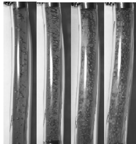
Fig. 3 – The observed flow patterns in water without addition of zeolite at 100 kPa.
