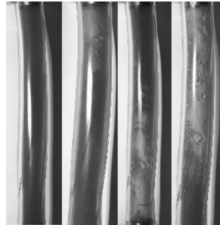
Fig. 5 – The observed flow patterns in suspension with addition of 10 \text{ g} \cdot \text{l}^{-1} of zeolite at 100 kPa.
