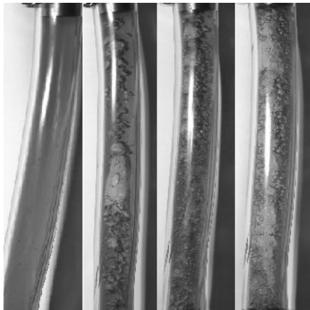
Fig. 4 – The observed flow patterns in water without addition of zeolite at 200 kPa.
