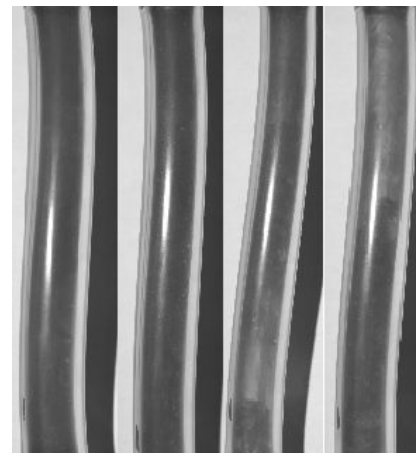
Fig. 6 – The observed flow patterns in suspension with addition of 20 \text{ g} \cdot \text{l}^{-1} of zeolite at 0 kPa.
