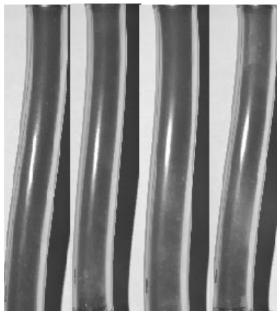
Fig. 8 – The observed flow patterns in suspension with addition of 30 \text{ g.l}^{-1} of zeolite at 0 \text{ kPa} .
