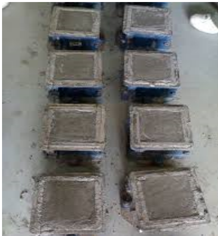
Fig2.10: cubes at the time of casting
