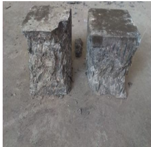
Fig2.12 : cubes after testing showing fracture
