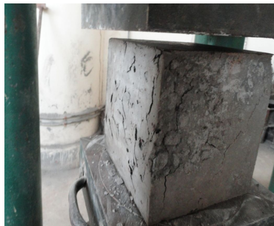
Fig 2.13 : Cube in Compression Testing Machine
