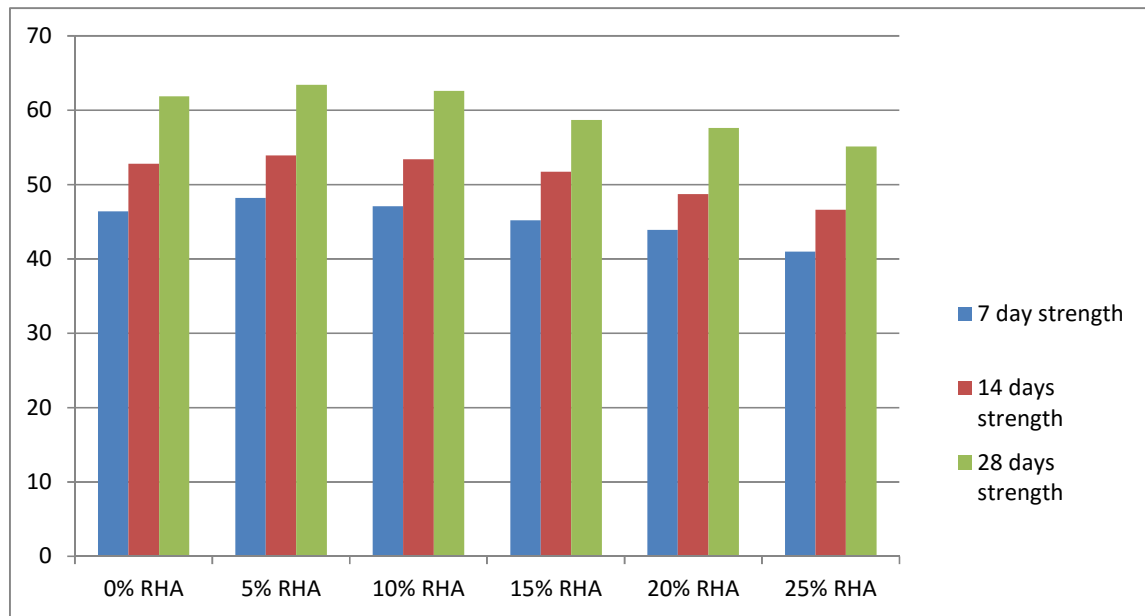
Fig2.16 : comparison of compressive strength of rice husk ash concrete
