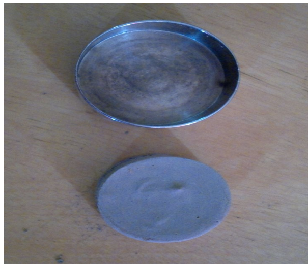
Figure4 : Shrinkage dish having wet soil pat
