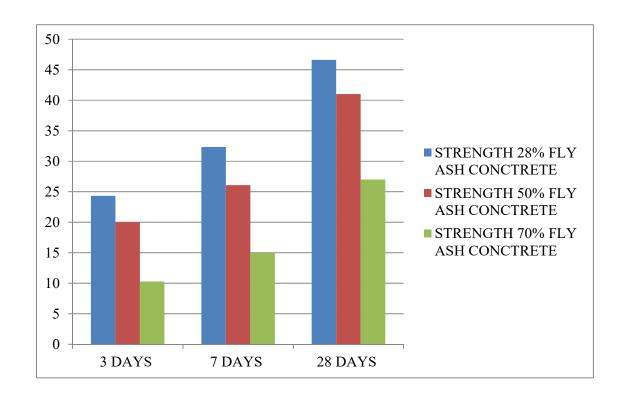
Figure 6.1: Compressive strength comparison of M40 concrete for 28%, 50% and 70% fly ash content.
