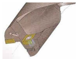
Fig.2 A model of collapsible tool with two cutting inserts for making holes
