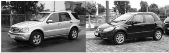
Fig.5 Larger SUV (left) introduced before 2003 (with frame chassis) and of small SUV (Right) after 2002 (with unibody)
