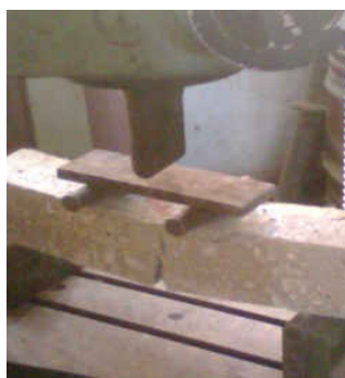
Fig.- Determination of Flexural strength of prism
