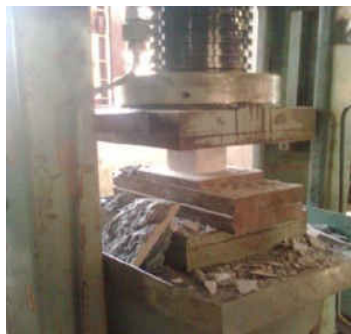
Fig. -Determination of compressive strength of cube
