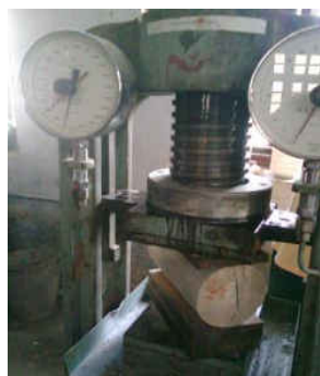
Fig.- Determination of splitting tensile strength of cylinder
