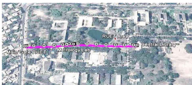
Figure 15. Track map obtained from the robot's movement (from RUET main gate to Central Library)
