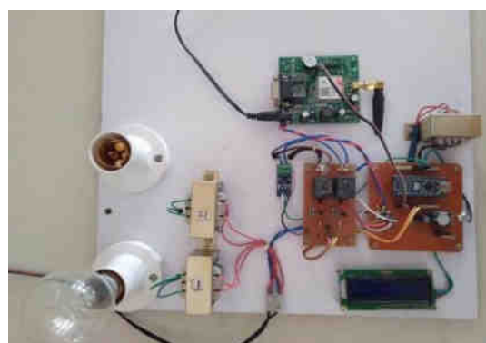
Figure 4: Working model of Load sharing of Transformer
