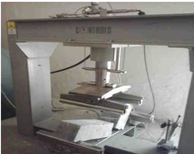
Figure 4.4 Test For Flexural Strength
