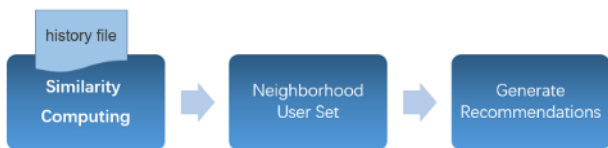
Figure 2 Collaborative filtering recommendation algorithm flow
